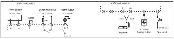
For a EMC-compatible installation it is necessary to connect the protective earth connecting terminal 3 via short way to control box or earth of the machine.
