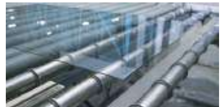
Detection of glass sheet on conveyor
