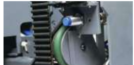
Drive-belt tension monitoring
